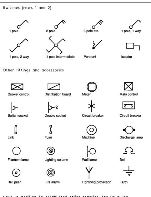
Note: In addition to established office practice, the following standards provide recommendations for drawing representations: BS EN 61082-2: Preparation of documents used in electrotechnology. Function oriented diagrams.
