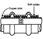
When the fitting is heated solder flows
