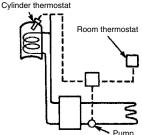
Two thermostats controlling the pump to give priority to hot water supply
