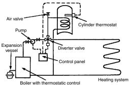
Use of diverter valve to give priority to hot water supply
