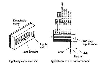
Refs: BS 5486-11 and 12, and BS EN 60439-3: Low-voltage switchgear and controlgear assemblies. Specifications.
