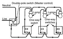
'Master' control wiring circuit
