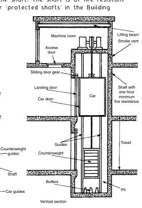
Refs: BS 5655: Lifts and service lifts. BS EN 81: Safety rules for the construction and installation of lifts. Building Regulations, Approved Document B3: Internal fire spread (structure).
