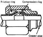
Manipulative compression joint on copper pipes
