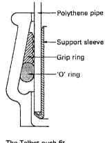
The Talbot push-fit joint on polythene pipes
