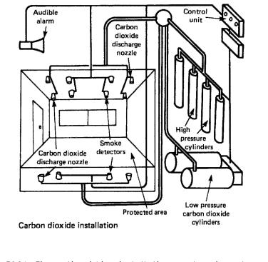
Ref: BS 5306: Fire extinguishing installations and equipment on premises, BS 5306-4: Specification for carbon dioxide systems.
