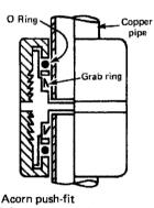
joint on copper pipes
