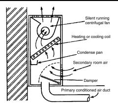
Section through a fan-coil room unit
