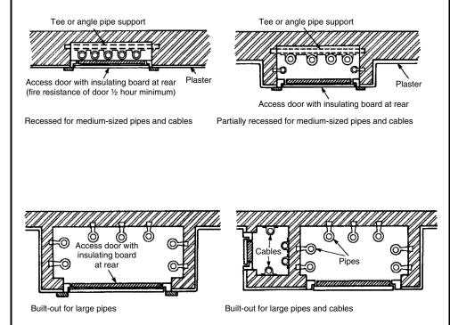
Refs.: BS 8313: Code of practice for accommodation of building services in ducts. Building Regulations, Approved Document B3: Internal fire spread (structure).
