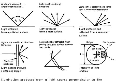
Illumination produced from a light source perpendicular to the surface:
