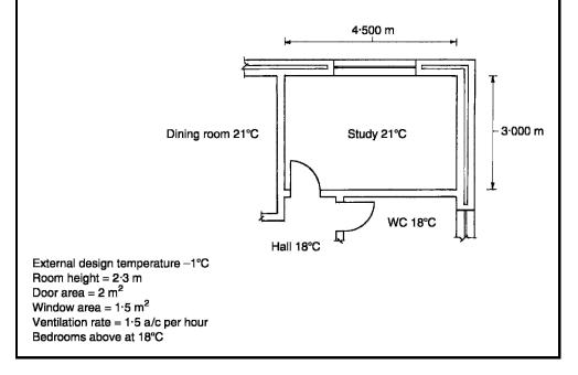
To determine the total heat loss or heating requirement for a room, it is necessary to obtain the thermal insulation properties of construction. For the room shown on the previous page, the `U' values can be taken as:
