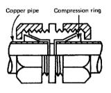
Non-manipulative compression joint on copper pipes
