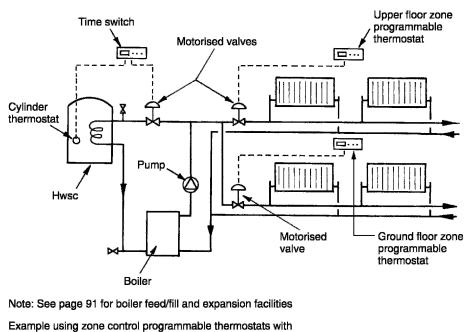
'wireless' (radio frequency signals) regulation of the boiler
